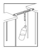
3) With the weight hanging, measure and record the change in length between the two lines (elongation).
